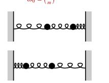
How does the middle spring effect this motion? The distances between the two masses remains fixed at all times, so the middle spring remains unstretched and hence does not do anything. Therefore, the above expression described the displacement of both masses, and each mass oscillates with the frequency  $\left(\frac{k}{m}\right)^{1/2}$ .
