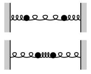
How can we calculate the frequency of oscillation? Consider the displacement  $x_l[t]$  of the left mass (since by symmetry  $x_r[t] = -x_l[t]$ ). The force on the left mass will be
